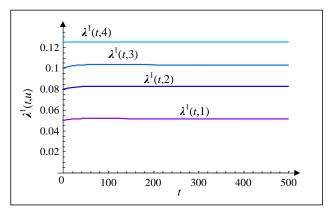
*Figure 8.* The graphs of the intensities of ageing of the car wheel system impacted by its components dependency
